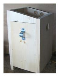
11. Position ROOF so its rear edge is even with BACK. Nail ROOF to BACK, SIDE, and FRONT.
