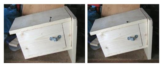
14. Screw VENT BLOCKER in place on upper SIDE. Right-hand screw is the pivot.
