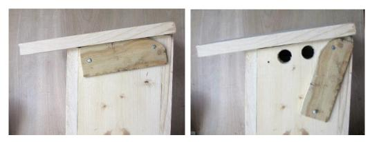
15. If you plan to mount the box on a metal pole, you can add hangers at this point. Mounting screws point outward from the inside of the box. We use round head machine screws, #8-32 x 2" long, with nuts and washers.
