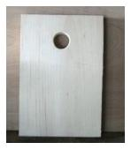
Drill two 7/8" or 1" **Vent Holes** in upper end of SIDE, about 3/4" from upper edge.
