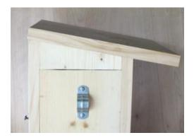
12. Fill gap between ROOF and BACK with wood filler.
