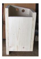
6. Drill pilot hole through FRONT into DOOR 3/8" up from bottom of FRONT and 3/8" in from FRONT's edge.
