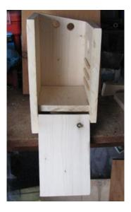
If Door hits Floor, remove nails and round off DOOR edges that hit the FLOOR. If this doesn't work you may need to reposition DOOR slightly down from flush with the FRONT.
